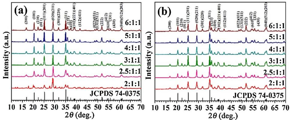
**Fig. 2.** XRD patterns of (a) LiMnPO<sub>4</sub> and (b) LiMnPO<sub>4</sub>/C.
