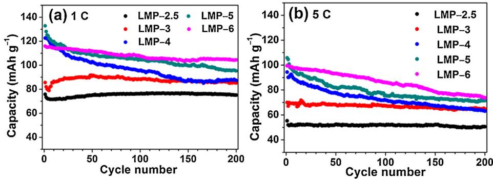
Fig. 6. Cycling performance of carbon-coated LMP-x at (a) 1C and (b) 5C.
