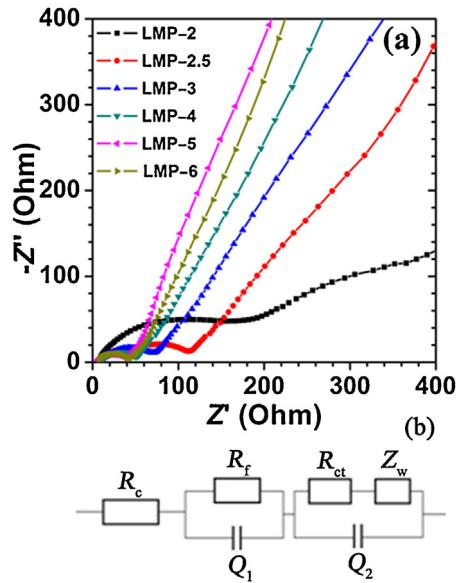
Fig. 8. (a) EIS plots of cells after 5 cycles at 0.05C and (b) corresponding equivalent circuit.
