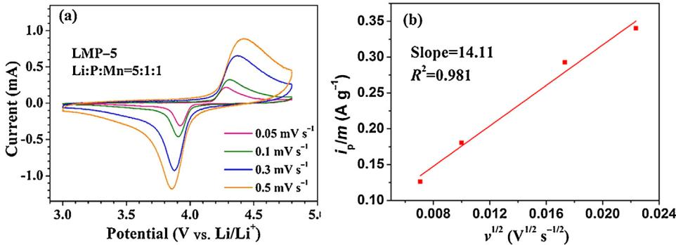
Fig. 7. (a) CV plots of LMP-5 and (b) linear response of cathodic peak current density as a function of square root of scan rate ( $R$ : goodness of fit;  $m$ : weight of active material on the electrode).
