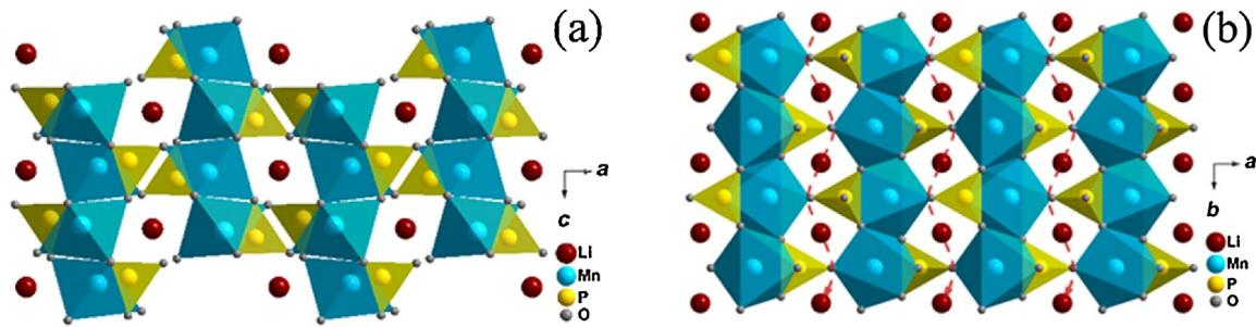
**Fig. 1.** (a) Crystal structure of olivine-type LiMnPO<sub>4</sub> projected along the [010] and (b) lithium-ion diffusion pathway parallel to [010].
