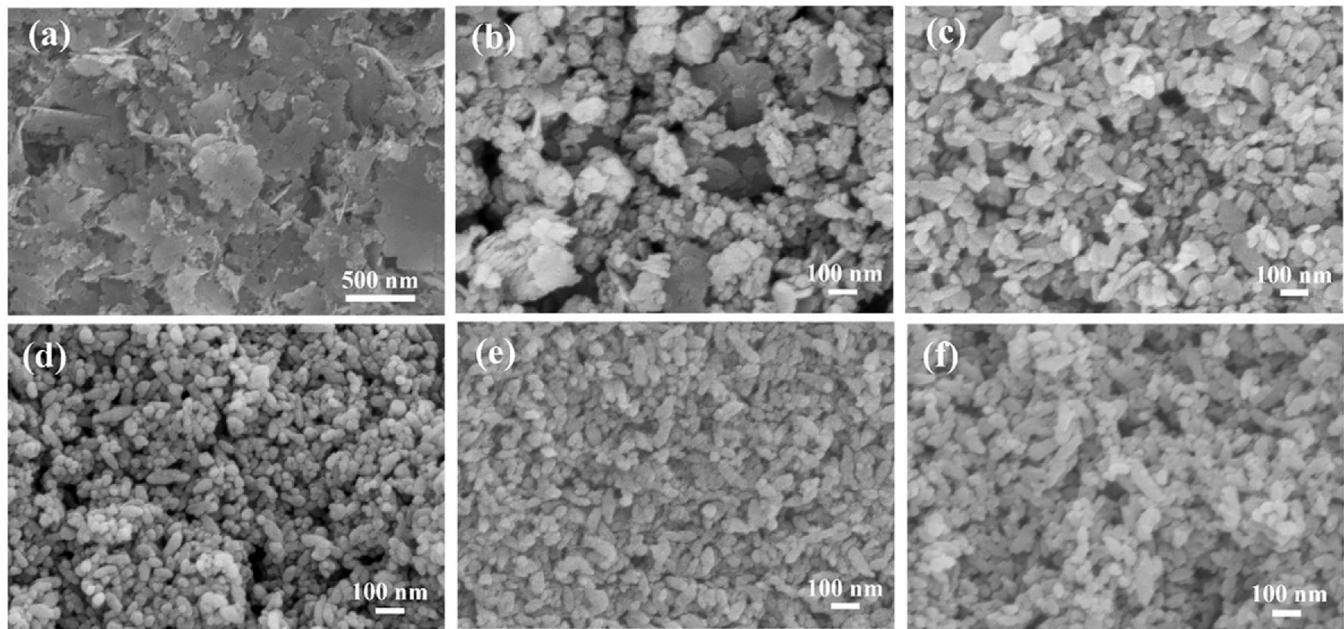
**Fig. 3.** SEM images of as-obtained LiMnPO<sub>4</sub>: (a) LMP-2; (b) LMP-2.5; (c) LMP-3; (d) LMP-4; (e) LMP-5; (f) LMP-6.
