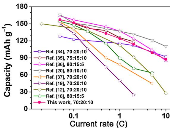
**Fig. 9.** Comparison of rate capability of sample and some typical LiMnPO<sub>4</sub>/C materials reported previously. The inset gives the LiMnPO<sub>4</sub>/conductive carbon/binder weight ratio.
