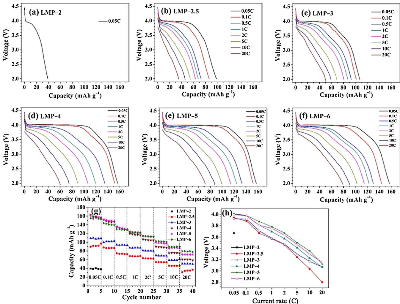
**Fig. 5.** Discharge profiles of (a) LMP-2, (b) LMP-2.5, (c) LMP-3, (d) LMP-4, (e) LMP-5, (f) LMP-6, (g) rate performance of LMP-x and (h) median voltage (voltage at half of discharge capacity) vs. current rate.
