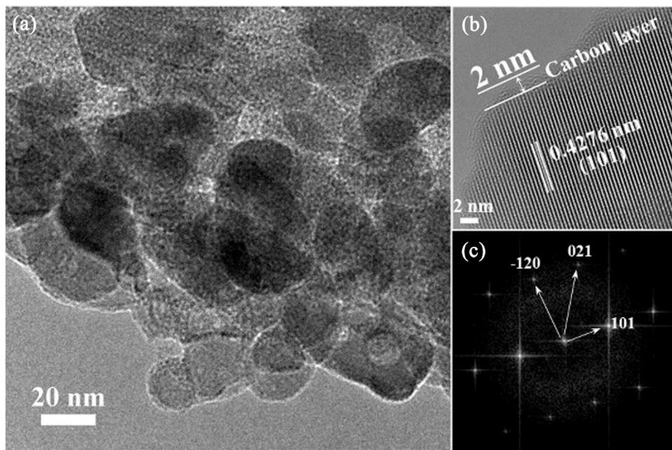
**Fig. 4.** (a) TEM, (b) HRTEM images and (c) SAED pattern of carbon-coated LMP-5.
